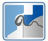
contamination. The double seaming method is usually used to seal metal containers. The seam is created in two operation steps.
