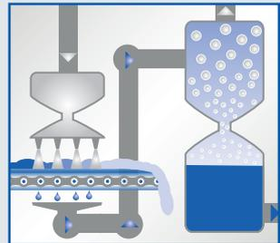
3. Refining: Neutralizing, degumming, bleaching, deodorizing
