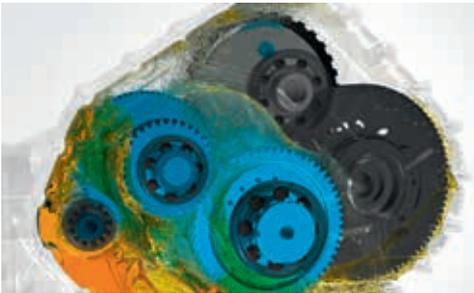
Simulation of the fluid flow in the high-speed transmission
