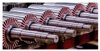
Electric motors component: rotor
