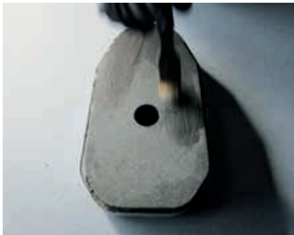
Cold coating of sealing surface of ceramic sliding ladle nozzle
