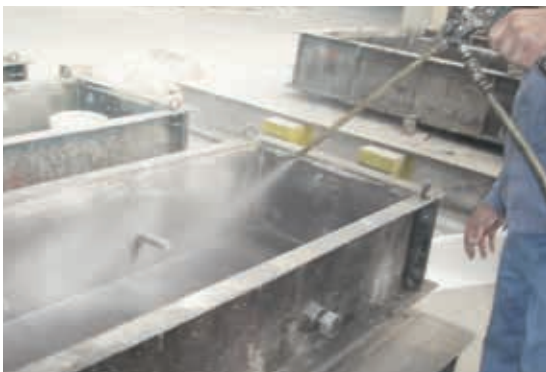
Spray-coating of a mould
