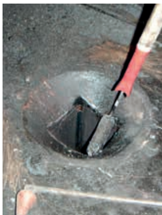
Continuous casting mould for billets: coating with fibre roller
