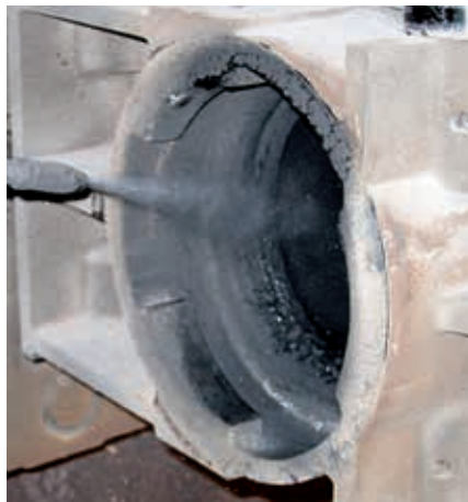
Hot-spraying, sealing surface sliding plate / exchangeable nozzle
