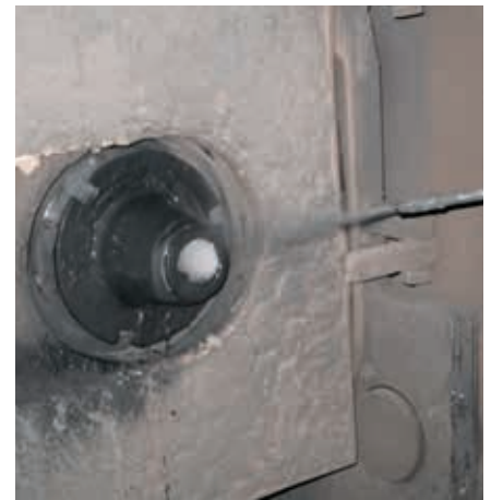
Hot-spraying, sealing surface exchangeable nozzle / ladle-shroud
