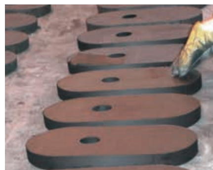
Manual surface coating of ceramic sliding plates
