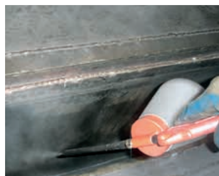
Surface spray coating of slab mould
