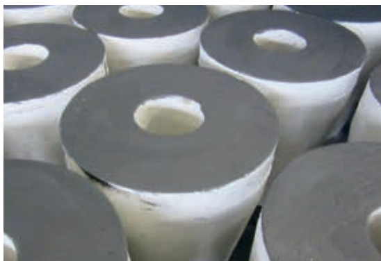
Cold coating of sealing surface of ceramic sliding ladle nozzle
