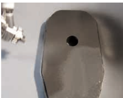
Surface coating (spraying) of linear sliding plate
