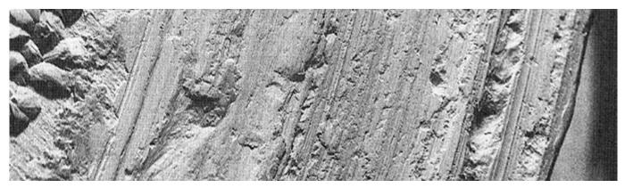
Lubrication with MoS<sub>2</sub> paste. Spindle surface after 35,000 motion cycles. Test aborted, as power consumption of motor too high (torque exceeded).
