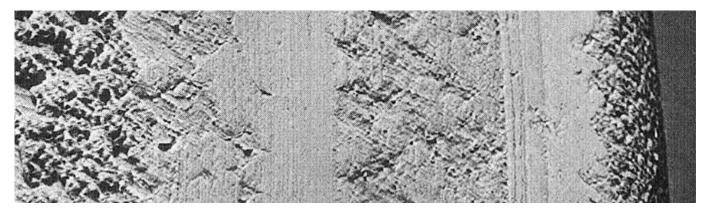
Lubrication with a paste that contains reactive white solid lubricants. Spindle surface after 500,000 motion cycles. Test aborted with spindle being fully intact.
