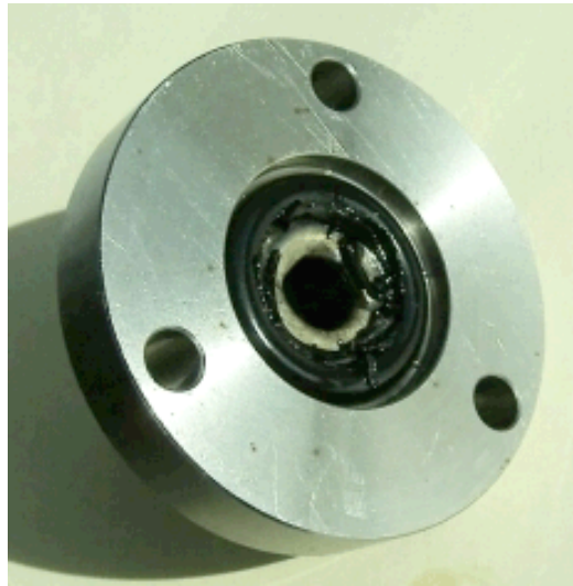
Figure 1 Dissolved O-ring made of Neoprene after 24h contact with R22
