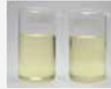
10% Naphtenic Oil ISO VG 68 90% RENISO UltraCool 68
