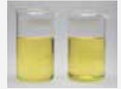
50% Naphtenic Oil ISO VG 68 50% RENISO UltraCool 68
