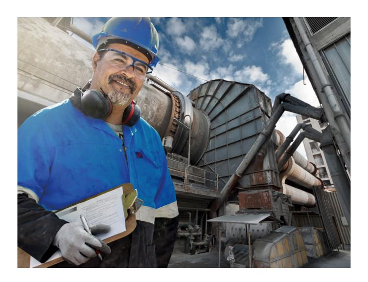
For drive units that are lubricated with CEPLATTYN, our service engineers carry out regular inspections over the entire service life. The service engineer takes extensive measurements (e.g. vibrations, tooth flank temperatures), which are recorded in the FUCHS LUBRICANTS INSPECTOR, an online documentation system, and is available to our customers at any time.
