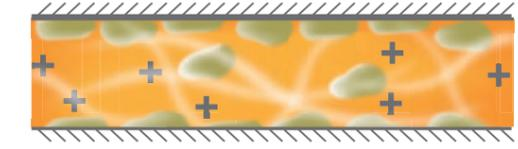
Conventional soap-based grease has a higher polarity than the additives. Consequently, a large amount of additive does not reach the metal surfaces.
