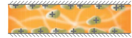
Grease based on functional soaps. The soap and the additives are intertwined - more additive reaches the surface, but a fair amount gets blocked in the middle.
